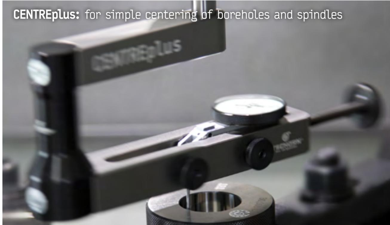
**CENTREplus:** for simple centering of boreholes and spindles
